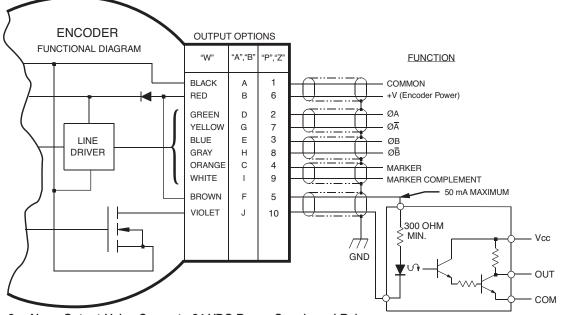
Example 2. Alarm Output Using Separate 24 VDC Power Supply and Relay.
